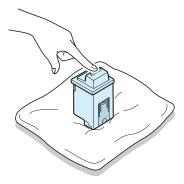
If you are cleaning a colour print cartridge, be especially careful to wipe the nozzles in only one direction so the colours do not mix.
